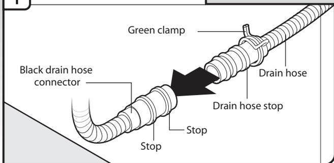
Place towel under drain hose to catch any water in drain hose. Place the small green drain hose clamp onto the small end of the drain hose. Push the new drain hose into the black drain hose connector up to the drain hose stop.
